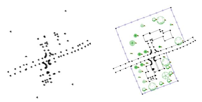
This is also important to describe topographic features, and can result in the creation of much more accurate surface models than without. The field crews is in the field and are the first and best witness to the characteristics of the land, where there are surface perturbations such as edges of embankments, flow erosions, and piles of dirt.
