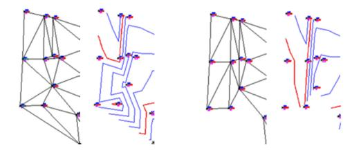
The difference in the interpretation of the points that were field collected to define an existing conditions surface in this example is significant. If the surface on the left is carried forward to the design and engineering analysis phase many things will be affected, such as earthworks, drainage, slope staking to name a few.
