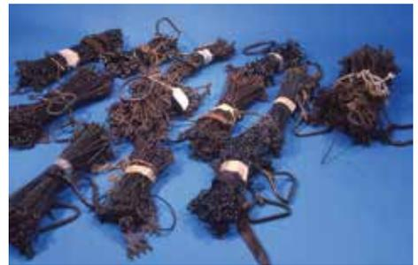
An assortment of chains: Gunter's Chain, 66 feet. A half-chain, 33 feet. Railroad or Engineer's Chain, 100 feet.
