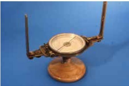
The standard American vernier compass by W. & L.E. Gurley. This form with vernier, outkeeper, sights, level vials, was made from about 1860 and remained in the Gurley catalogs into the 1930s. It attached to either a tripod or Jacobs Staff.
