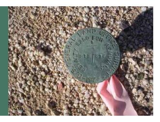
often cover, disturb, or remove monuments. Road millings regularly remove all or portions of the monument while overlays make the monument difficult, if not impossible, to access. In Salt Lake County, a new road surface might be several feet above an existing brass cap monument. Additionally, chip seal and crack repair activities have permanently sealed monument ring and lids.
